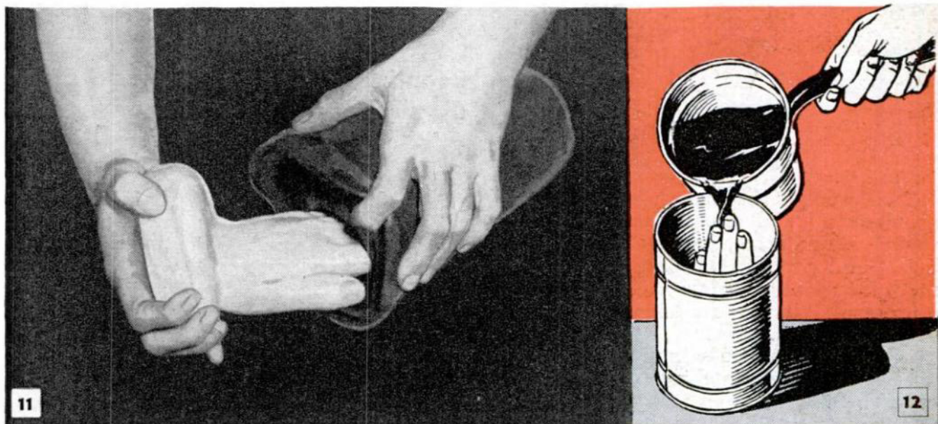
Master and subsequent castings are extracted from mold by stretching it. Open-end can provides mold form
